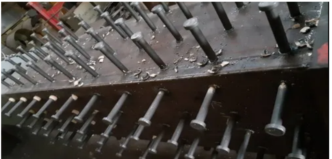
Shear Stud welding at Workshop
